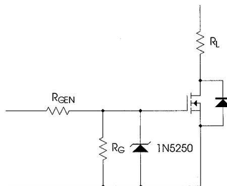
Figure 28. Zener Diode to Prevent Excessive Gate-Source Voltages
