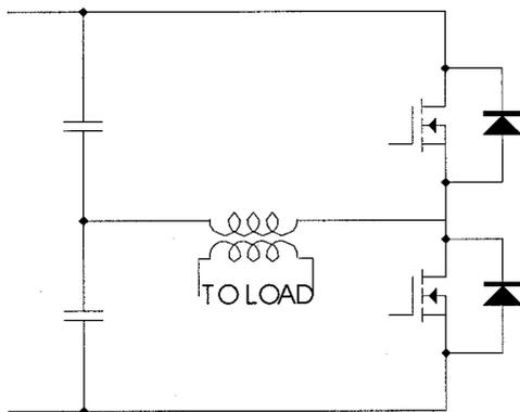
Figure 24. Half-Bridge Configuration
