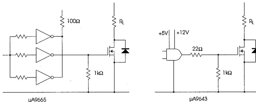
Figure 21. Interface ICs Used to Drive Power MOSFETs
