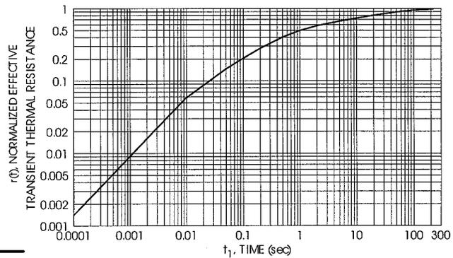
Figure 12b. Transient Thermal Resistance Curve for NDS351N
