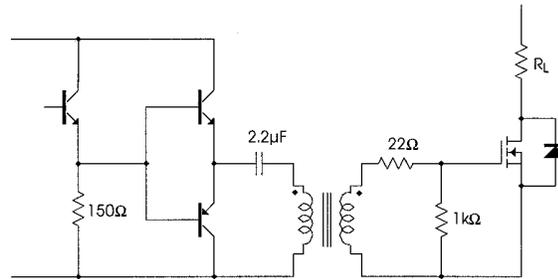
Figure 27. Emitter Follower Driver with Speed-Up Capacitor
