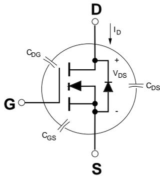
Figure 6a. MOSFET Capacitance Model for Power MOSFET
