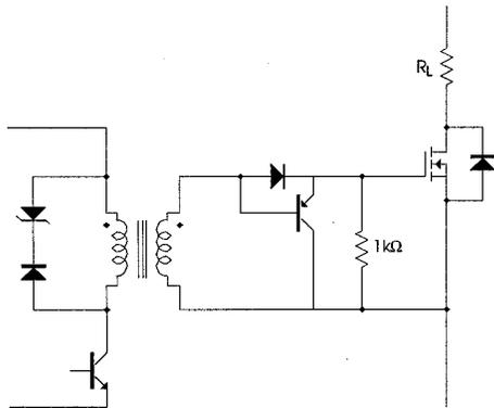
Figure 26. Improved Performance at Turn-Off with a Transistor
