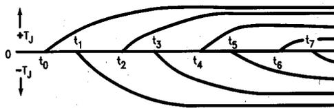
Figure 13c. Junction Temperature Response to Individual Power Pulse
